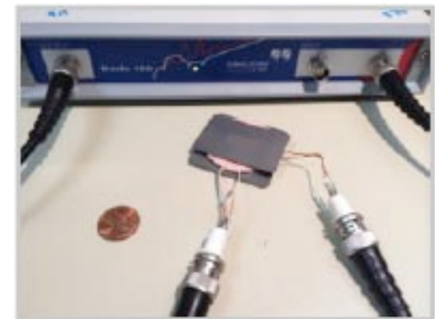
Typical 5 W coils Connected to a VNA
